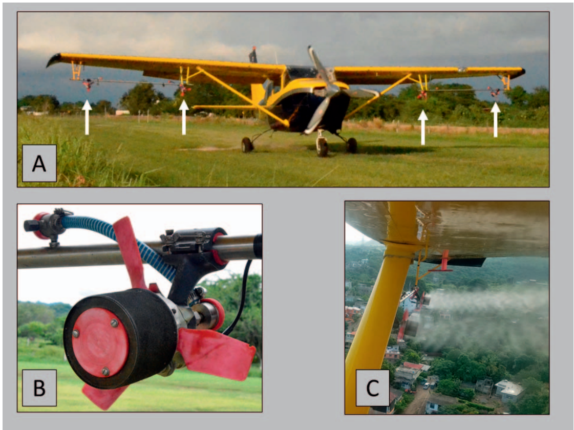
Fig. 3. (A) Aircraft employed in the trials with arrows indicating the 4 nozzles, (B) the rotary atomizer mounted under a wing, and (C) the aerial view at the time of application.
